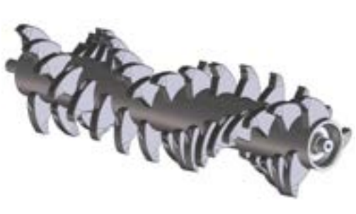
Forestry rotor with fixed chisels for branches and shrubs up to ø10-12 cm
