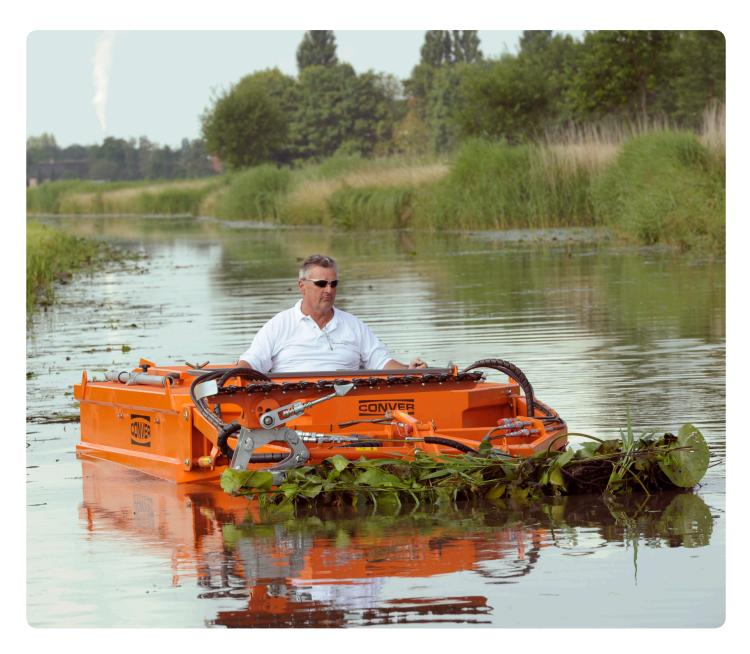
Conver mowing boats are specially developed for removing plant growth from embankments and the flow-profiles of waterways. The well thought-out design and chosen components make the mowing boats reliable in all conditions. Moreover, the C420 performs a variety of jobs. It can be equipped with a trailing knife unit, embankment cutting unit, push frame and T-front cutter. Like all our mowing boats, the C420 can be easily and safely transported using the Conver boat trailer.
